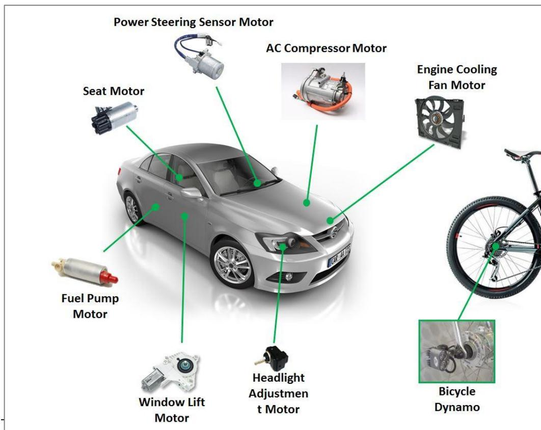
Some of the motors in a modern automobile that can utilize permanent rare earth magnets with little to no Dysprosium.
