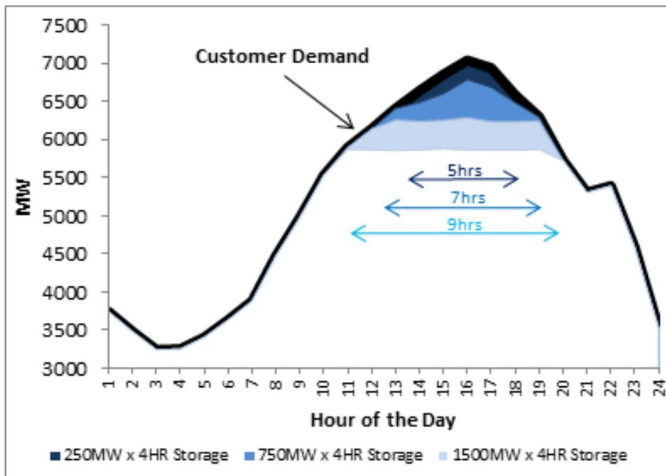
This chart shows that more batteries with longer duration and lower capacity are required at each step to reduce the peak. At some point, it is not technically or economically feasible to continue to use storage to shift energy from off-peak to on-peak periods.
