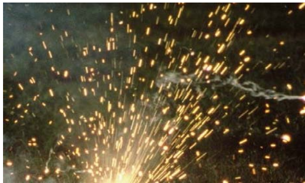
Figure 5 – Incandescent particles emitted from an arcing electric conductor.
