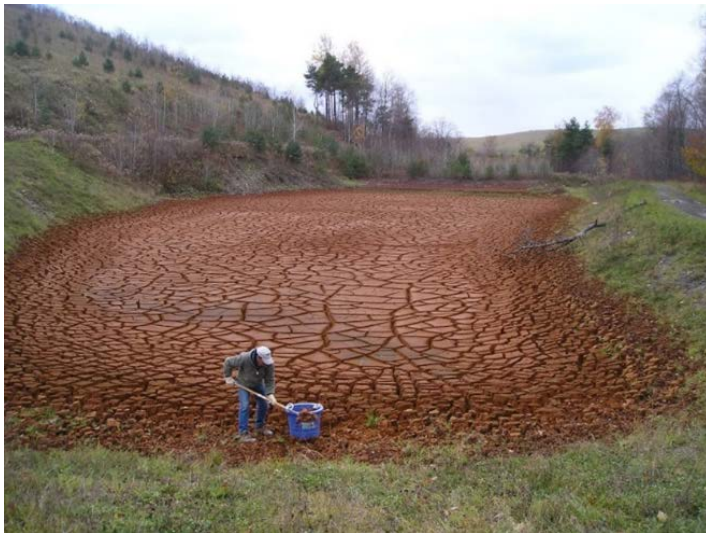
Figure 3. Typical AMD sludge storage cell at a West Virginia coal mine. The contained rare earth value of this small cell is estimated at $325,000.
