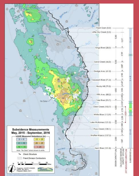
The graphic shows the areas of subsidence along the Friant-Kern Canal and the degree to which canal capacity has been compromised from its original design.
