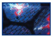
one of the lightest solids ever made and have the highest heat resistance of any material tested. They also are fireproof and extraordinarily strong — able to support more than a thousand times their own weight. As a result of their heat resistance, aerogels are outstanding candidates for insulation in buildings, vehicles, filters and appliances.
