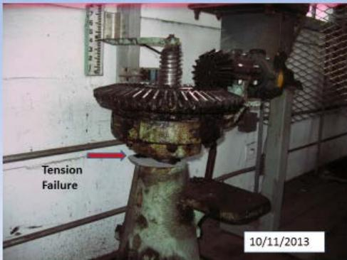
Debris gets pinched between the headgates and the concrete floor as the gates are lowered at the end of the irrigation season and causes damage such as sheared gate operator pictured at left and bent gate stem in picture below.
