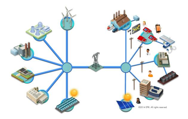
Many of the innovations are occurring at the edge of the distribution system, the far right-hand side, where customers connect to the power system. Because the power system is interconnected, changes that occur at the edge can impact the entire power system, including the rest of the distribution system, the transmission system and central generation on the far left-hand side.
