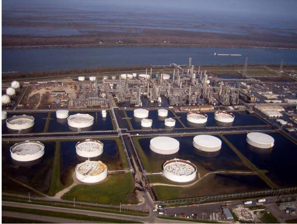
**Figure 9.** Over one million gallons of oil spilled from a storage tank damaged by Hurricane Katrina. The U.S. Coast Guard estimated at least 9 million gallons of oil were spilled from combined Katrina-Rita damage to offshore and coastal facilities. Photograph by U.S. Environmental Protection Agency.
