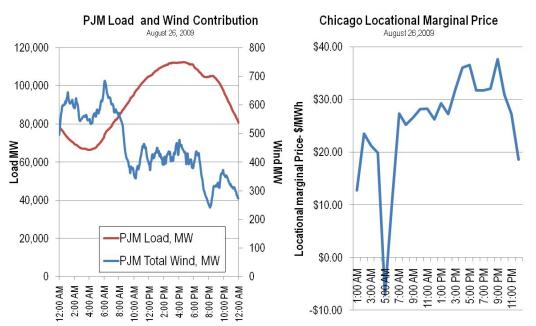
Figure 5: PJM Load and Wind Resources as of August 2009
