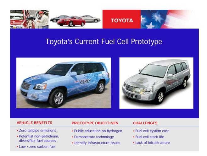
Let me conclude with a brief description of Toyota's Fuel Cell Hybrid Vehicle ... another evolution of our basic hybrid drive technology. This vehicle is based on the previous-generation Toyota Highlander Hybrid SUV but with a fuel cell, of Toyota's own design and manufacture, in place of the Highlander's gasoline engine. The combination of an advanced fuel cell system with our hybrid drive technology more than doubles the vehicle fuel efficiency with zero tailpipe emissions.
