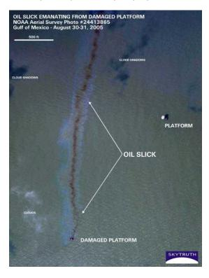
Figure 8. NOAA aerial survey photo showing oil leak from Katrina-damaged platform. Analysis by SkyTruth.
