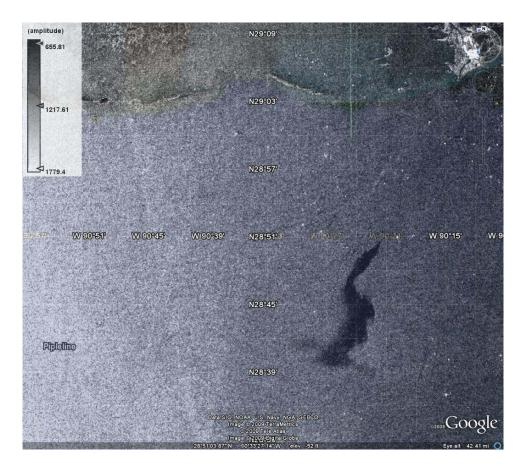
Figure 12. Satellite radar image showing 15-mile-long oil slick caused by Eugene Island Pipeline break in July 2009. Image courtesy of NOAA/NESDIS.
