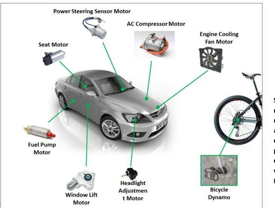
Some of the motors in a modern automobile that can utilize permanent rare earth magnets with little to no Dysprosium. A separate technology trend is the continuing migration from tri-phosphor fluorescent lighting to LED lighting. Tri-phosphor lighting utilizes several relatively scarce rare earths, such as Terbium, Europium, and Yttrium. This continuing shift to LED lighting is already helping to soften demand, and increase the availability, of HREEs like Terbium and Yttrium.
