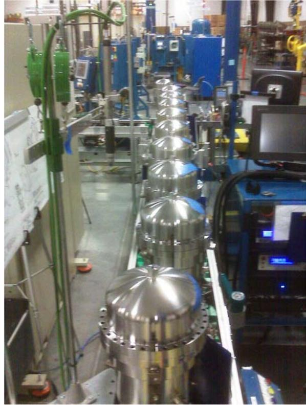
Stirling engines on assembly line
